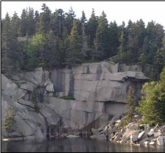
Fig. 4: Hurricane's main quarry face, showing sheeting of the granite.
