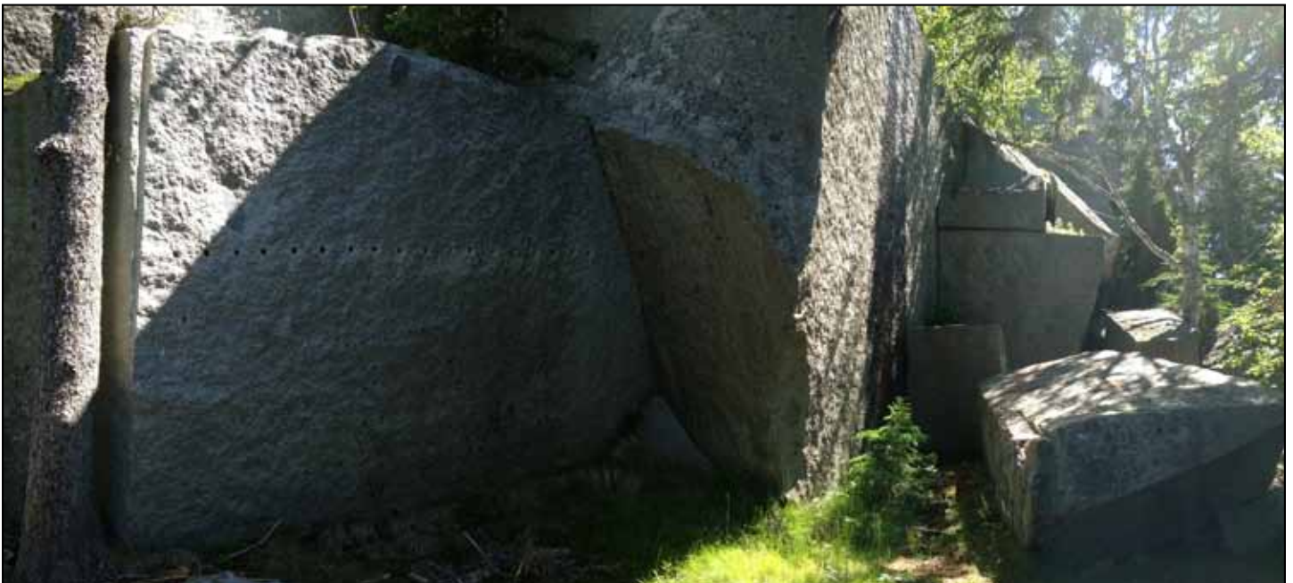
Fig. 7: Blocks of granite partially quarried from the main face on Hurricane Island. Note perforations from steam drills.
