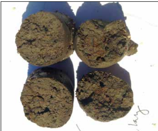
Fig. 33: Redoxomorphic features (note reddish areas) on broken column samples of lower clay
