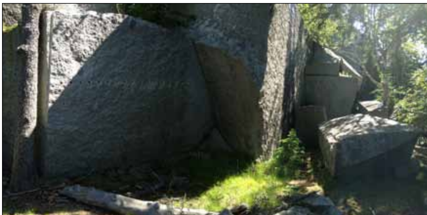
Fig. 23: Left: Blocks of granite partially quarried from the main face on Hurricane Island. Note perforations from steam drills. Right: Remains of the flywheel constructed to send steam power to the quarry face.
